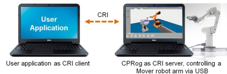
Robots without embedded control, e.g. the Mover robots, can also be commanded using the CRI interface.
