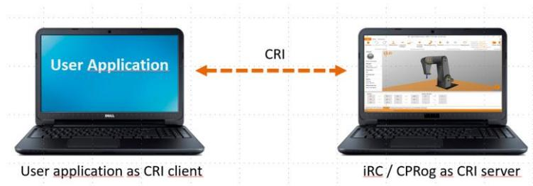
For the development of applications, the user application can interact with iRC igus Robot Control / CPRog. The commands are then executed by the simulated robot arm.
