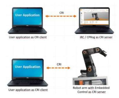
For the development of applications, the user application can interact with igus Robot Control / CPRog. The commands are then executed by the simulated robot arm.
