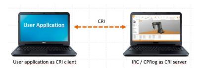
For the development of applications, the user application can interact with iRC igus Robot Control / CPRog. The commands are then executed by the simulated robot arm.
