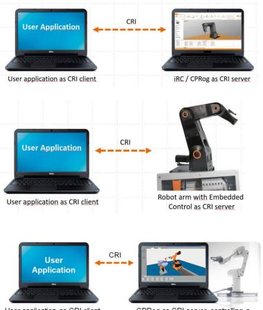
For the development of applications, the user application can interact with iRC igus Robot Control / CPRog. The commands are then executed by the simulated robot arm.
