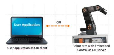
With the same interface a robot arm or gantry with embedded control can be addressed.
