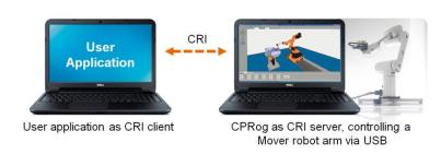
Robots without embedded control, e.g. the Mover robots, can also be commanded using the CRI interface.
