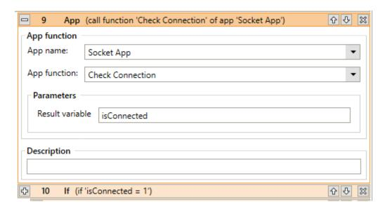
Check connection sets a variable value to 1 if a connection is established (i.e. messages can be sent out). Otherwise it sets the variable to 0.
